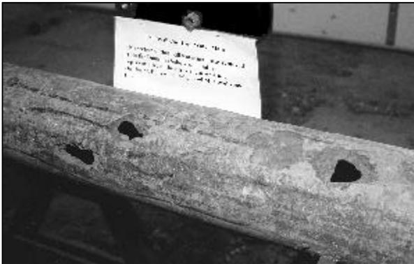
This old water main, removed from the Dunhurst subdivision, is an example of why the Village has embarked on an extensive replacement program to update the existing water-delivery system.
